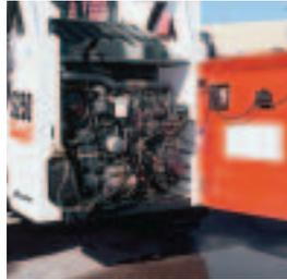
checks and fills, filters and battery. And unlike other brands, the lift arms need not be raised to service the machine. Shop time is spent repairing, not gaining access.
