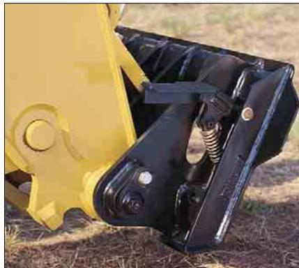
**Manual Coupler.** The TH210 utilizes a manual quick coupler using the same interface as the Caterpillar Skid Steer Loader.
