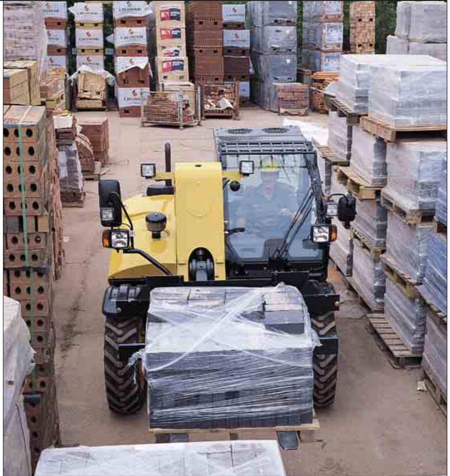
**Steering Modes.** The compact telehandlers offer three steering modes, (circle, two wheel and crab steer) to allow an operator to easily position the machine in small, confined areas. Steering modes are selected by using the steering mode switch in the operator's compartment. An indicator light in the cab illuminates when the wheels are properly aligned.
