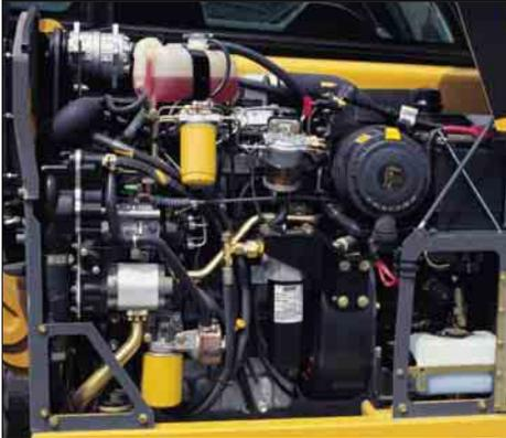
**Ease of Access.** The TH210 utilizes a side mounted engine design, which provides easy access to major service points. Regular maintenance is important in ensuring a long, productive machine life and also helps minimize downtime on the job. The complete service schedule can be found in the Operation and Maintenance Manual that accompanies the machine.
