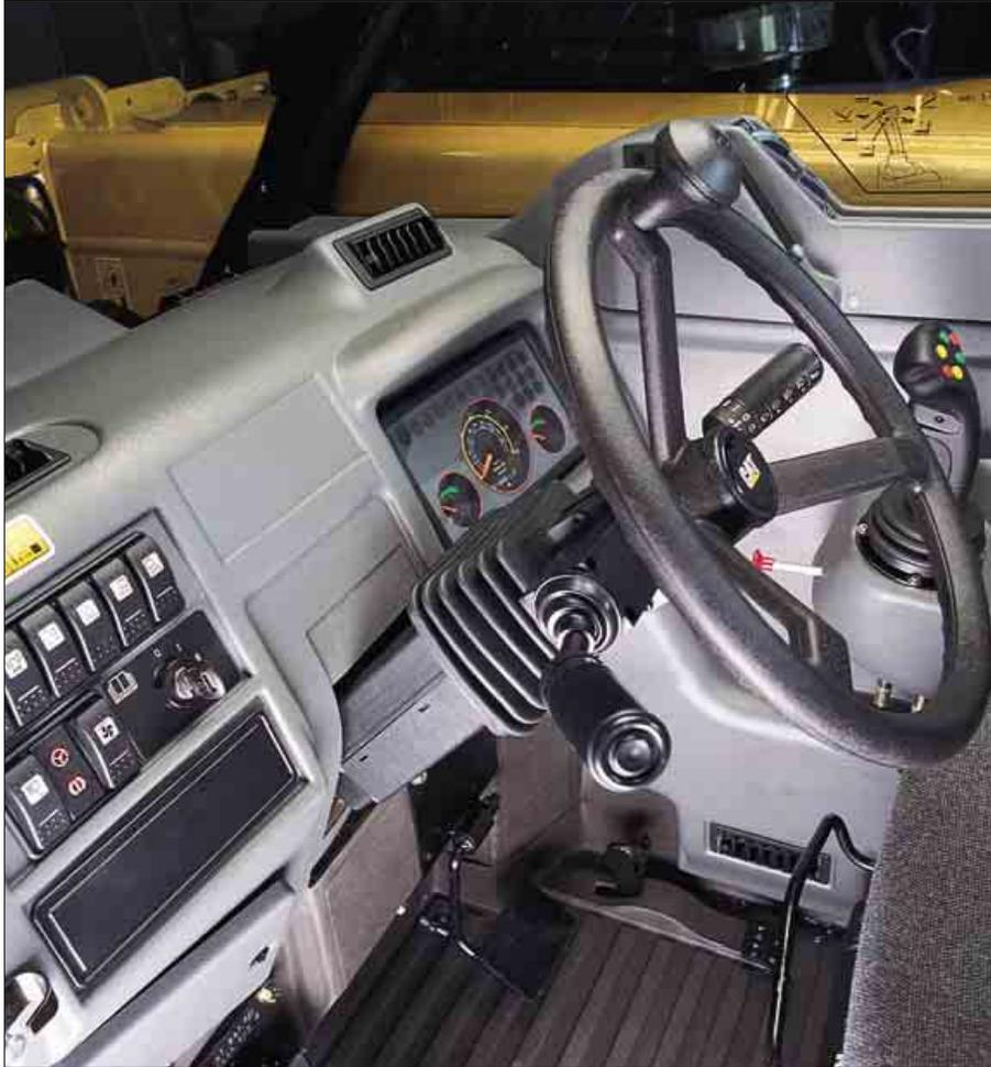
**Enclosed Cab.** The TH210 is equipped with an enclosed cab allowing the operator to work comfortably, with air conditioning available as an option. The cab structure has been designed and certified to provide falling object and rollover protection (FOPS/ROPS).
