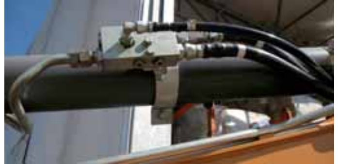
Safety valves included in the Safe Handling kit
