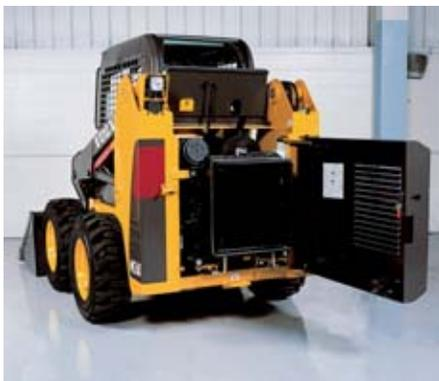
The rear door swings open wide and the top engine cover flips up to give you access to all key service points. The drive chain access plate can be removed to get to key chaincase components. And a hydraulic sight gauge with a level indicator is mounted on the hydraulic tank, inside the rear door. In addition, corrosion-resistant pins and self-lubricating bushings require minimal lubrication, saving time, and money.
