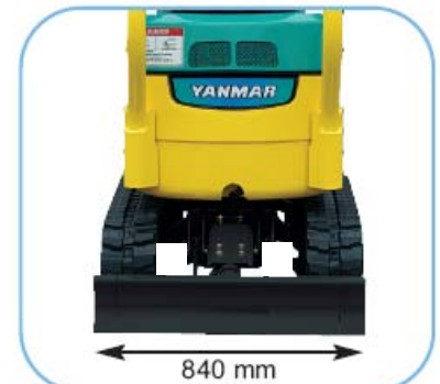
Extended undercarriage for better stability
